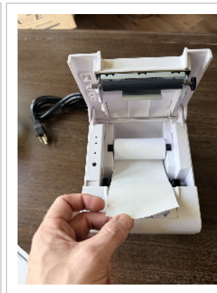
Fig. 5c — Insert spindle through roll; coated side up.
