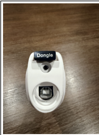
Fig. 4c — Scanner underside: dongle location.
