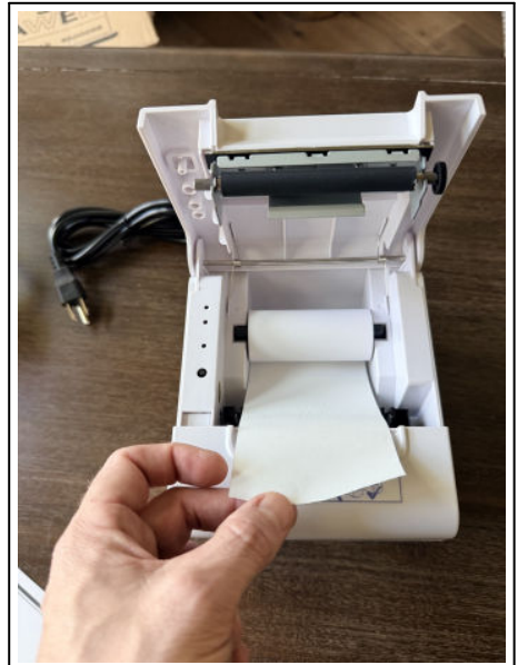
Fig. 5c — Receipt paper & spindle dropped in.
