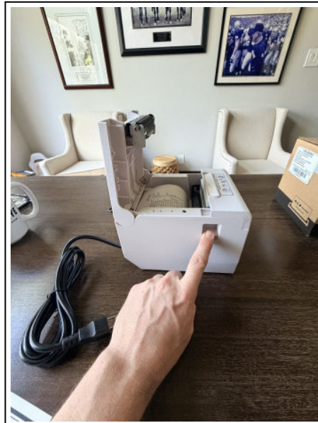
Fig. 5b — Press the side button to open the lid.
