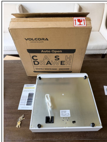
Fig. 6b — Underside: RJ11 port for printer trigger.
