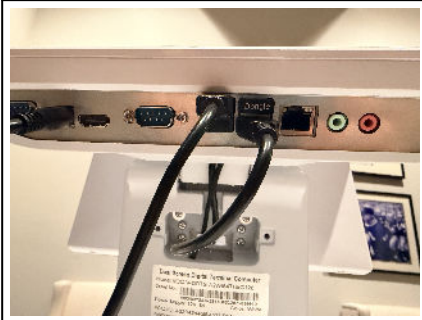
Fig. 4e — Terminal underside: all cables and dongles connected.
