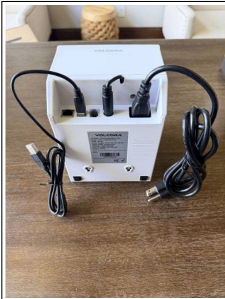
Fig. 5a — Printer rear: USB-B data and DC power ports.
